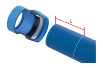
The required insertion depth [L] must be marked on the pipe end before installation (see table). Use drinking water-approved lubricants and apply a thin layer exclusively (!) on the gasket.
