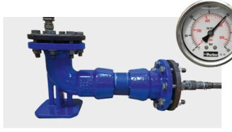
The mechanical advantages of the cast iron fittings are evident on the test bench where they can withstand testing pressures well beyond typical operating conditions.
